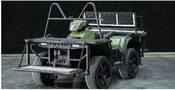
1. Camera Quad Bike ATV Car Rig
