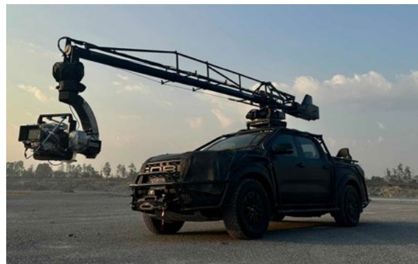
2. Scorpio Arm with tracking vehicle and Remote Head Stabilizer
